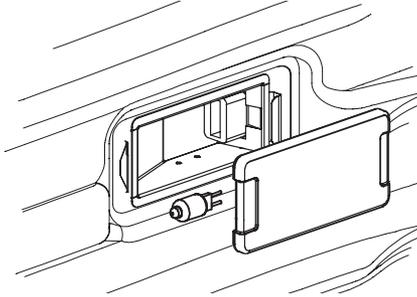
**NOTE:** To avoid damage or decreasing the life of the new bulb, do not touch bulb with bare fingers. Wear cotton gloves or use a tissue when replacing the light bulb.
