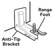
Making sure the anti-tip bracket is installed:
